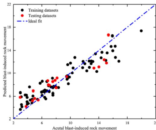
Figure 7 Actual rock movement measurement vrs predicted values by WOA-GP. Source: (Yu, Shi, Zhou, Gou, et al., 2021)
